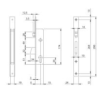
Mortice lock for metal frames, LATERAL LOCKING, operating with European profile cylinder.
