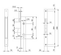
Mortice lock for metal frames, LATERAL LOCKING, operating with European profile cylinder.
