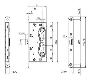
LOCK FOR LEFT- AND RIGHT- HANDED FIRE RESISTANT PANIC EXIT DOORS (EXTERNAL HANDLE). 1 lateral point, latchbolt only. Internal: latchbolt operated by the panic exit device, by the handle or by the key.
